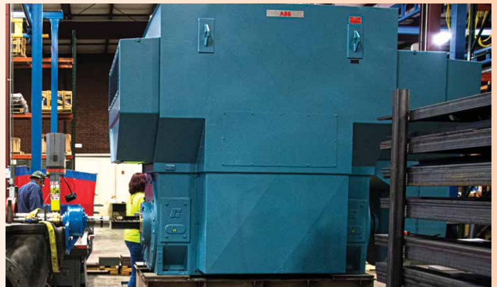
A 1000HP, roughly 17,000 lb. ABB motor and pump were sent to our Proshop
