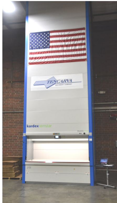
The new Vertical Lift Module in the Greensboro Warehouse maximizes floor space for product and parts storage.
